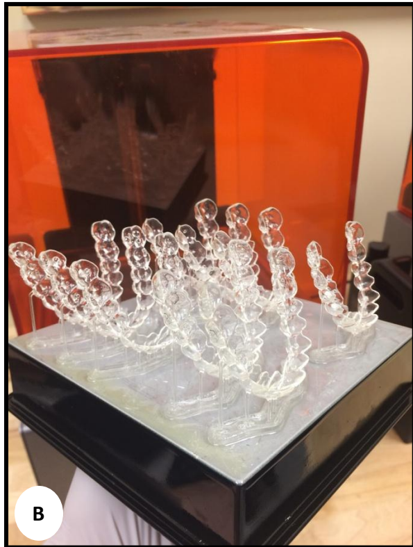
Figure 5. 3D printed retainers. Printed retainers for Models 1, 2, and 3 while still connected to the printing platform (A). Printed retainers for Models 1, 2, and 3 after removal of printing platform from the SLA printer (B).
